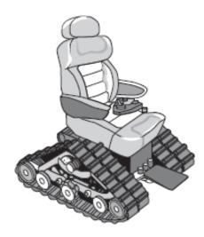
The Tankchair is a special type of "wheelchair." This <u>unusual</u> chair uses tracks instead of tires or wheels, just like a tank. It is a custom off-road wheelchair that can go almost anywhere outdoors. The Tankchair can go through streams, mud, snow, sand, and gravel. Its rubber tracks and powerful electric motors make it possible to even climb steps!
